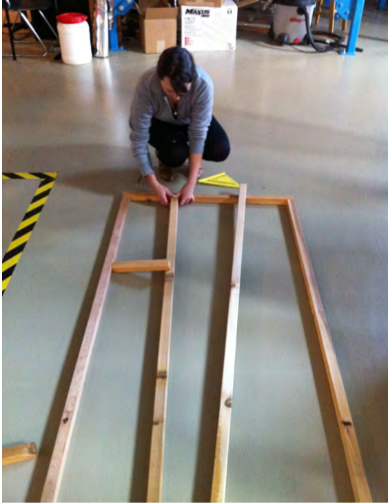
Figure 1: Cedar Backing Construction
